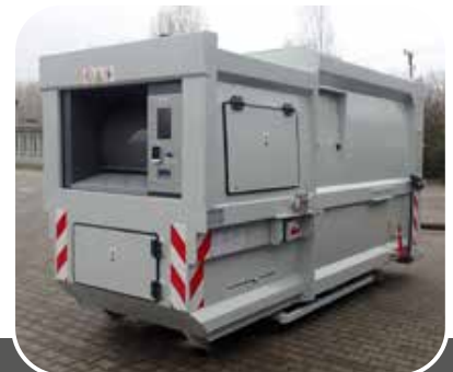
Compactor with weighing system
